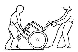
FIGURE 2.4 Method 2 - Wheelchair Without Step Tubes
